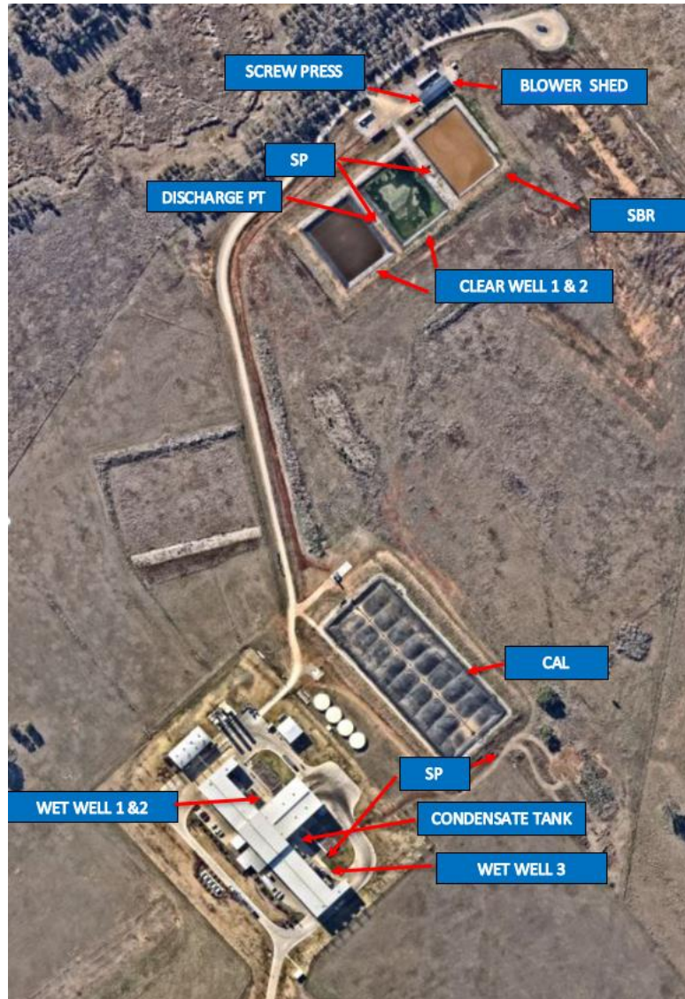
Figure 1: Waste Water Key Infrastructure
