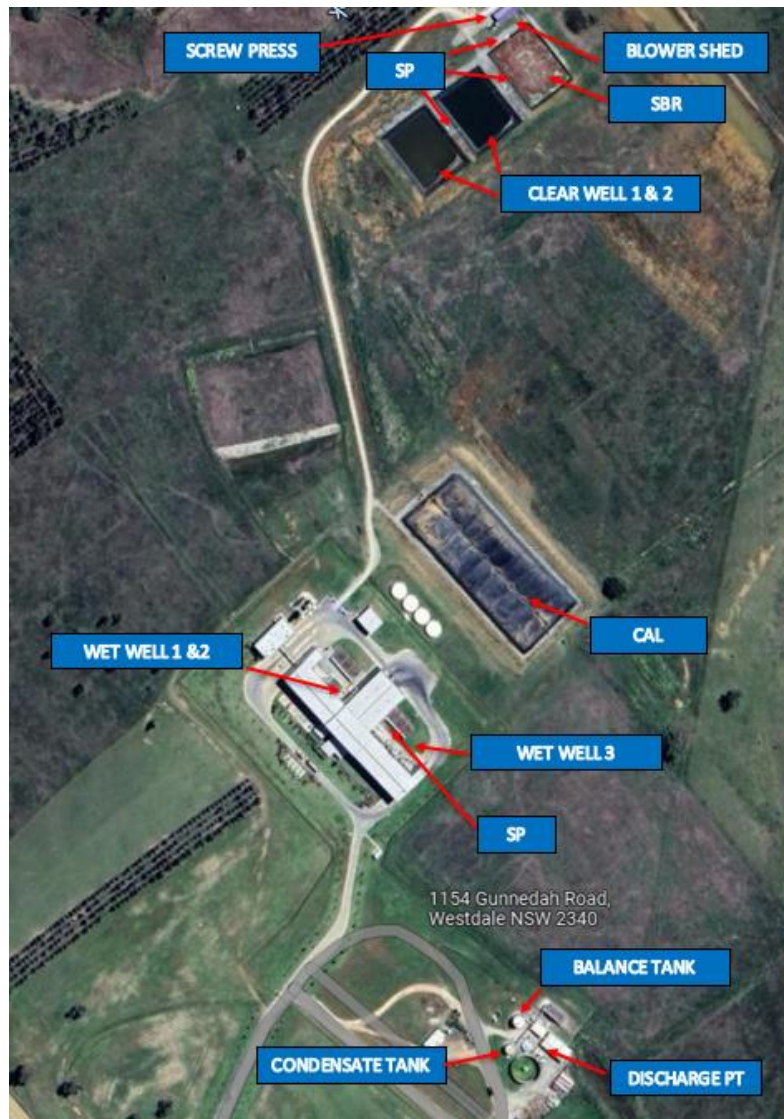
Figure 1: Waste Water Key Infrastructure
