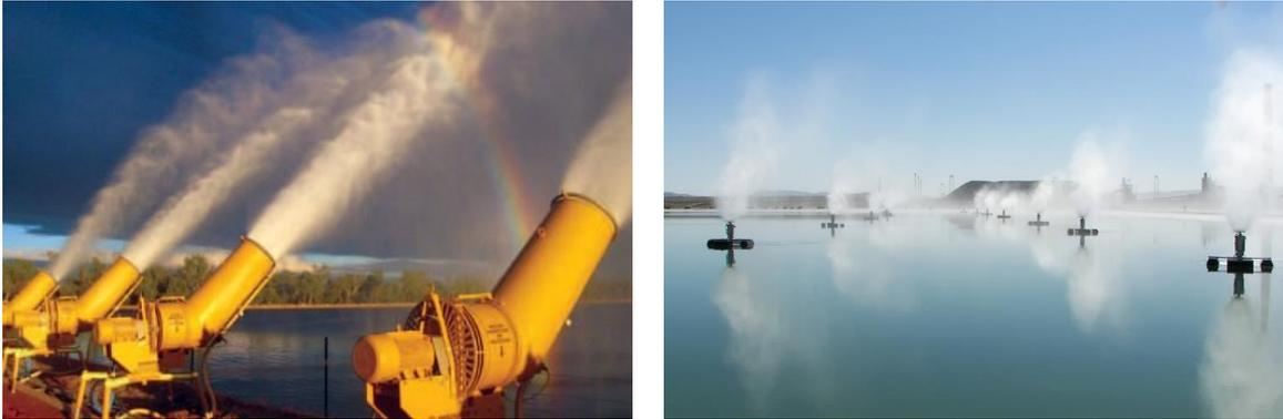
Figure 1 - Images of Typical Accelerated Evaporation Processes
